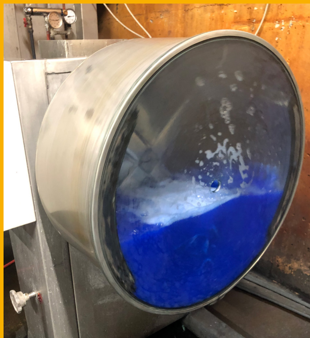
Dyeing of fish leather after tanning with sustainable formic acid. Source: Nordic Fish Leather
